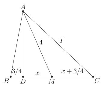
By the Pythagorean theorem on  $\triangle ADM$  and  $\triangle ADC$ , it follows that  $AD^2+x^2=4^2$  and  $AD^2+(2x+\frac{3}{4})^2=T^2$ . Subtracting these two equations,  $(2x+\frac{3}{4})^2-x^2=T^2-4^2$ , which for T=5 simplifies to  $3x^2+3x-\frac{135}{16}=0$ , or  $x^2+x-\frac{45}{16}=0$ . This factors as  $(x+\frac{9}{4})(x-\frac{5}{4})=0$ , so  $x=\frac{5}{4}$ .
